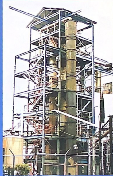
A set of three distillation columns for producing "clean" ethanol.
