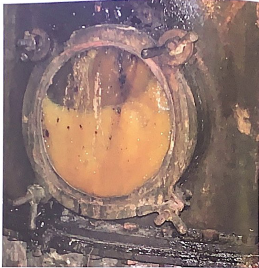
The removable porthole of one of the sections between two plates of a copper column still in operation. Volatile vapours pass upwards with the heat; the watery, depleted dead wash passes downwards.
