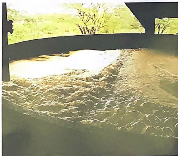
"Live wash" in an open fermenter: carbon dioxide bubbles up while the sugars are being converted to ethanol. Some of the ethanol evaporates and gives a "heady" atmosphere downwind!
